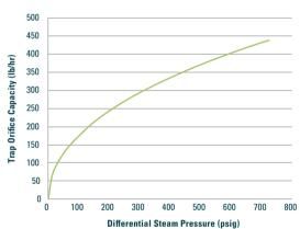
Maximum discharge capacity for Flanged Opal Trap at saturation temperature.\*
