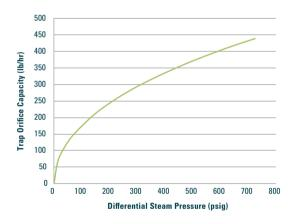
Maximum discharge capacity for Emerald Trap at saturation temperature.\*
