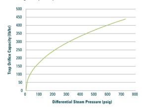
Maximum discharge capacity for Opal Trap at saturation temperature.\*
