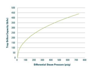
Maximum discharge capacity for Quartz Trap at saturation temperature.\*
