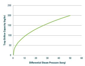
Maximum discharge capacity for Ruby Filter Trap at saturation temperature.\*
