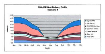
The initiative recovers 100,638 mmBTU of heat per year. This volume is guaranteed through a performance contract with Johnson Controls. Johnson Controls are responsible to design, build, operate, monitor and maintain the system under contractual agreement. If the agreed volume of heat is not delivered, Johnson Controls is obligated by guarantee to pay Minas Basin a fixed amount for each mmBTU of the deficiency.
